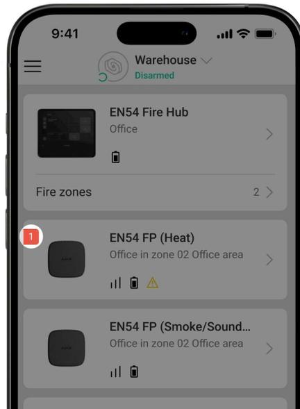
When an EN54 FireProtect (Heat) Jeweller fault is detected, an Ajax app displays a fault counter on the device icon. All faults are indicated in the device states. Fields with faults are highlighted in yellow. Also, faults are displayed in the **Control** tab of the CIE display. More details about the fault can be found in the **Event center** or **Fire zones** tabs of the CIE.
